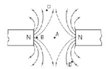
The diagram shows the lines of magnetic force between two north magnetic poles. At which point is the magnetic field strength greatest?
